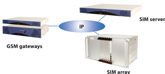
The QuesCom distributed architecture for Service Providers consists of 3 entities the SIM array (SIM bank), the SIM server that provides an intuitive web-based interface to manage the SIM cards & GSM gateways.
