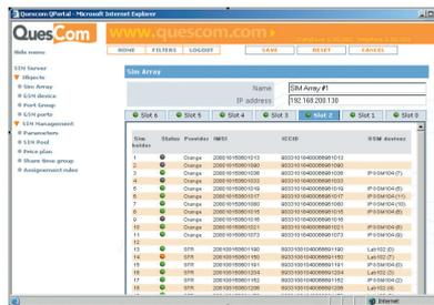
According to the time of the day, GSM gateways are loaded with the most adapted SIM cards. A comprehensive web-based interface enables to manage the SIM allocation based on intuitive rules.
